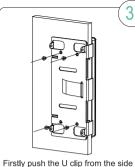
of the glass door and screw up 4 fixing screws.
