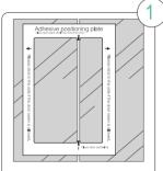
After cleaning the glass, attach the fixing template of adhesive plate to the door (door seam is aligned with door seam line of template door)
