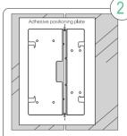
Remove the adhesive tape from the adhesive plate, and attach it to the middle blank and press it tightly (the small feet of the adhesive plate are close to the door tightly)
