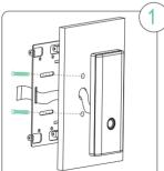
According to the size requirements please open holes on the door and fix the main lock through cables and screws, and finally fix the back panel by screws.
